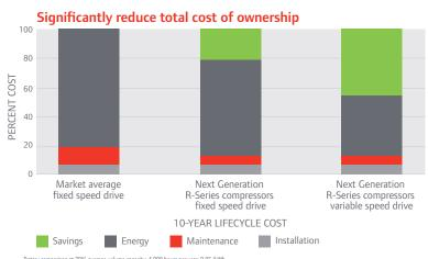
Rotary comparison at 79% average volume capacity; 4,000 hours per year;  $0.05/k \ensuremath{\mathbb{W}h}$
